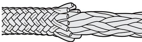
**Double Braid (Page 89)** - Double braided rope is, as the name implies, a braided core surrounded by a braided sheath. The inner and outer braids are generally designed
