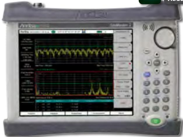
**ANRITSU SITE MASTER S331E COMPACT HANDHELD CABLE AND ANTENNA ANALYZER**
