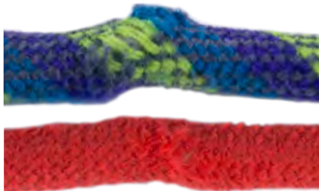
Pictures above showcase damaged rope cores and frayed/abraded sheath
