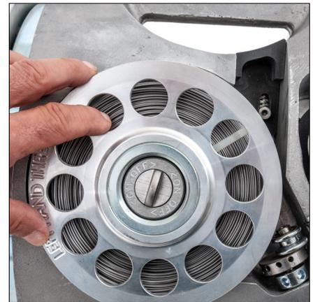
6. Install the wire reel cover and thread (CCW) completely onto the reel until snug against the wire coil. It is important to ensure that the reel cover is tight against the wire coil to prevent the lashing wire from "snagging" on itself.
