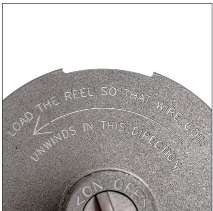
4. Slide the lashing wire coil over the hub and onto the reel making sure that it spools out to the rear of the lasher as shown by arrow.
