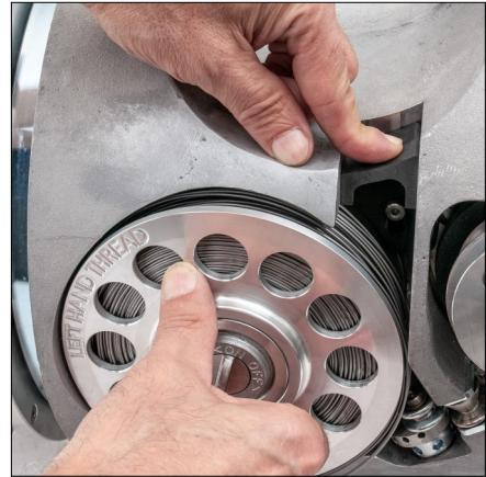
9. The reel brake can be depressed into cutout on rear flange to hold the reel stationary as you tighten the reel cover.
