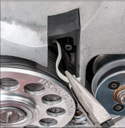
8. Remove the remaining cable tie.
