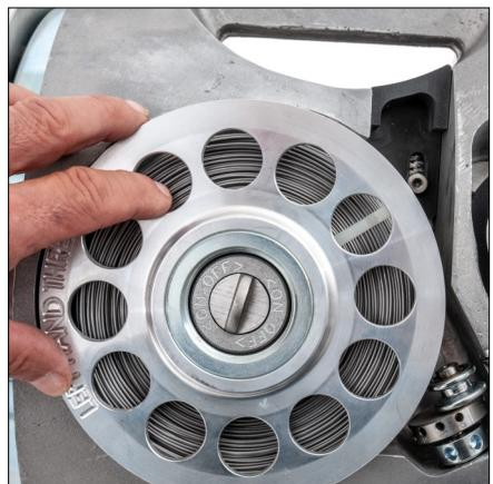
6. Install the wire reel cover and thread (CCW) completely onto the reel until snug against the wire coil. It is important to ensure that the reel cover is tight against the wire coil to prevent the lashing wire from "snagging" on itself.
