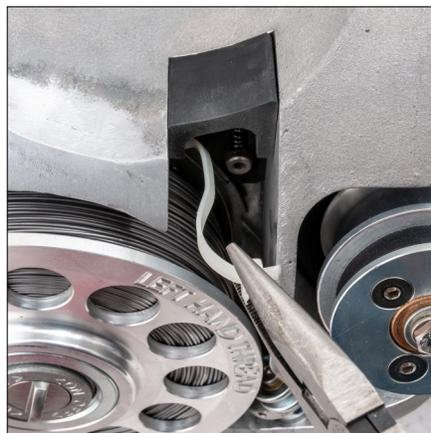
8. Remove the remaining cable tie.
