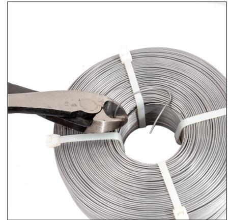
3. Cut the looped end of the wire on the inside diameter of the wire coil. This step will help in the loading of the coil onto the hub and subsequent steps.
