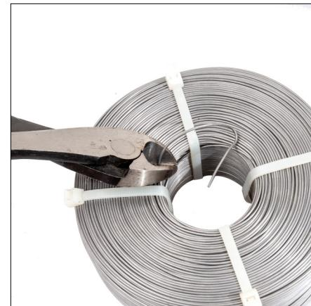
3. Cut the looped end of the wire on the inside diameter of the wire coil. This step will help in the loading of the coil onto the hub and subsequent steps.
