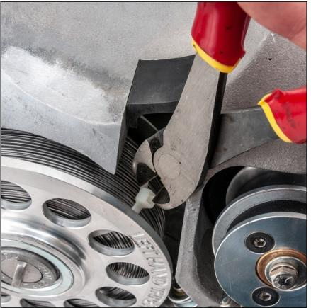
7. Cut and remove the remaining cable tie and then continue to snug the reel cover against the wire coil ensuring a tight fit.
