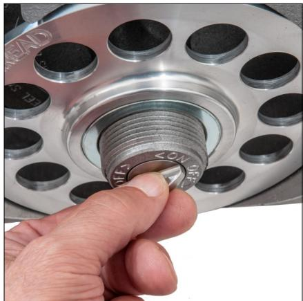
1. The reel can be loaded while attached to the lasher or by removing the reel and loading it on a flat surface. The reel is removed by turning the knob on the hub and the reel cover is re-
