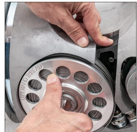
9. The reel brake can be depressed into cutout on rear flange to hold the reel stationary as you tighten the reel cover.
