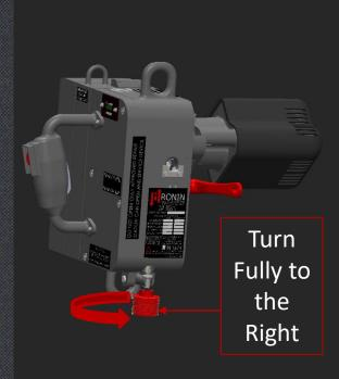
Step 2: Insert an approved Static Line Rope (10 mm to 13 mm diameter) into the rope inlet hole. Push until it stops. TAP the thumbwheel once, while pushing the rope. Continue pushing the rope and tapping the thumbwheel, until 8-10 inches (20-25 cm) of rope has fed into the system.
