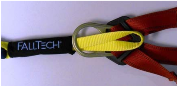
Fig. A-4 – Making Web-Loop Connections
