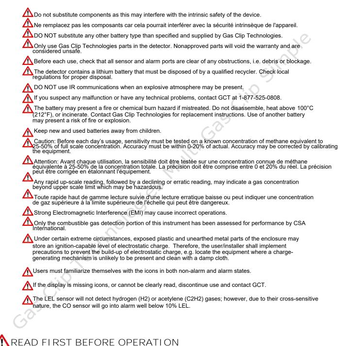
Gas Clip Technologies (GCT) Multi Gas Clip Simple (MGC-S) detectors are personal safety devices designed to detect the presence of specific toxic gases: carbon monoxide (CO), hydrogen sulfide (H<sub>2</sub>S), oxygen (O<sub>2</sub>) and combustible gases/Lower Explosive Limit (LEL). Before operation, ensure that you have been properly trained on the use of the equipment and the appropriate actions to take in the event of an alarm condition.
