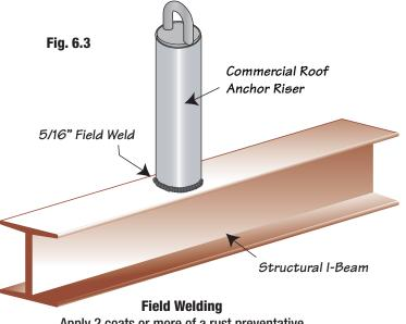
Apply 2 coats or more of a rust preventative coating to all field welds and raw risers
