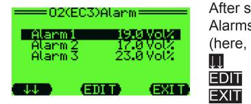
After selecting the sensor menu point Alarms the following reading is displayed (here, for an  $O_2$  sensor):
