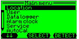
Left key (Uscroll down) Middle key (SELECT) select menu point Right key (DETECT) back to detection mode
