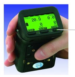
Turn the G450 on in an environment known to be free from gases and / or vapors.
