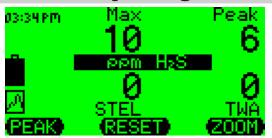
During peak mode (activated by pressing the left key **PEAK**), peak values can be monitored and displayed. The display shows an animated symbol in the bottom left corner.
