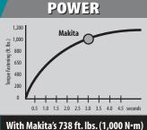
of torque it only takes 3 seconds to seat a 1-3/16" bolt
