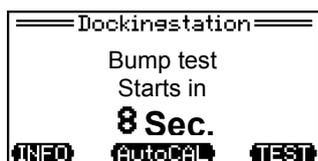
Bump test automatically starts after 10 seconds
