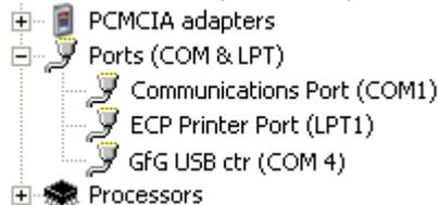
7. This is the COM port number for the GfG DS400/404 Docking Station. When setting up the DS400/404 software this COM port will need to be assigned.
