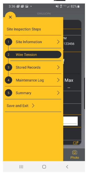
At this time, the mobile device will attempt to wirelessly connect to the Quick Check-T selected in the Devices screen. If unsuccessful, ensure the Quick Check-T is powered on and visible in the **Devices** menu.
