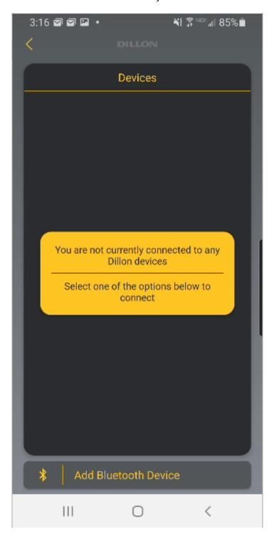
5. The mobile device will now scan for powered on Quick Check-T's in the area and display them in the Devices List.
