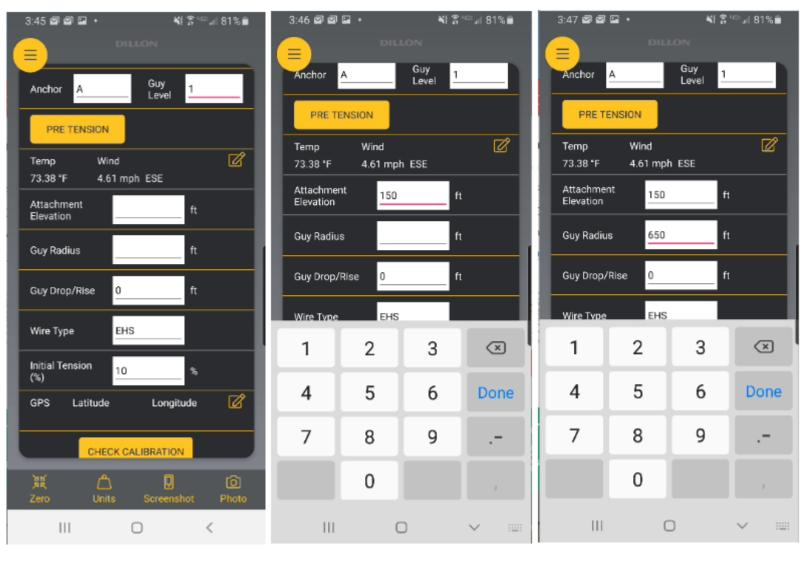
At this time, you can also change the Wire Type from Extra High Strength (EHS) to Bridge Strand (BS) and set the Initial Tension%.
