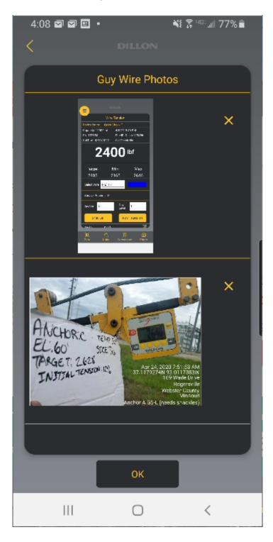
6. By pressing any of the store records, the Wire Tension screen will be brought up with the selected Anchor and Guy Level settings already loaded. The intent is the user will periodically go to the Stored Records screen to see a summary of the guy tension measurements and jump to the selected Anchor and Guy Level to complete the Post Tension measurements after adjustments have been made.
