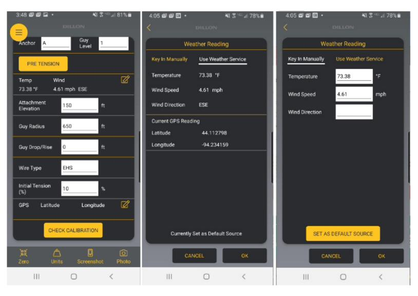
13. Press the **OK** button when finished to return to the Wire Tension screen.
