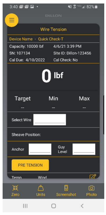
5. The Target, Min & Max Tensions will be blank. Once the Tower and Guy Wire measurements are entered, these will be calculated.
