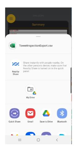
The exported file is a CSV (Comma-Separate Vales) file that can be imported into a spreadsheet program like Microsoft Excel. The file contains all the Site Information, Wire Pre Tension (Pre Tn) and Post Tension (Post Tn) readings, and text descriptions of the Maintenance Log.
