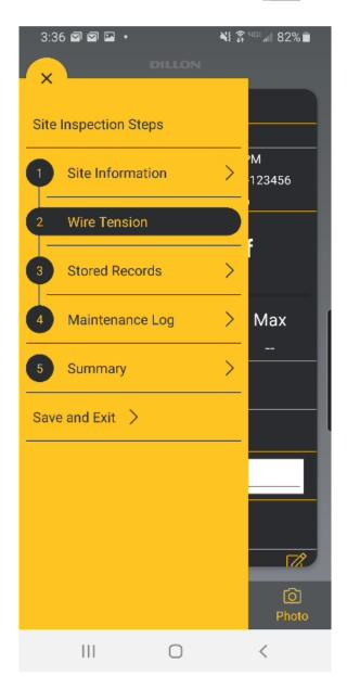
At this time, the mobile device will attempt to wirelessly connect to the Quick Check-T selected in the **Devices** screen. If unsuccessful, ensure the Quick Check-T is powered on and visible in the **Devices**.
