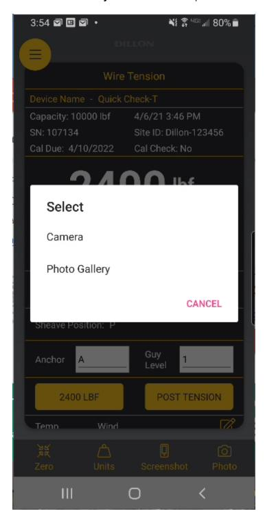
16. After the Guy Wire has been tensioned to target, the **Post Tension** button can be pressed to store the final tension to the Anchor and Guy Level selected. The value of the Post Tension reading will show where the Post Tension button used to be.
