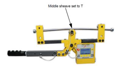
6. Clamp the Quick Check-T onto the calibration rod. Be sure the rod is riding in the center groove of all three sheaves, as shown above.
