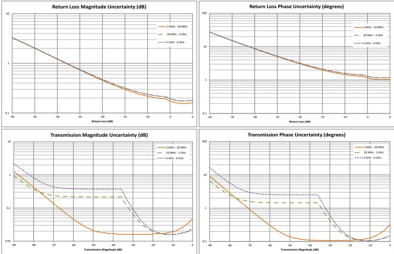
1. Full 1-path, 2-port forward path calibration with isolation, high power, 10 Hz IFBW, no averaging, 10 minute warm-up. TOSLK50A-20, TOSLK50A-20 calibration kit. Reflection and Transmission Tracking are typical.
