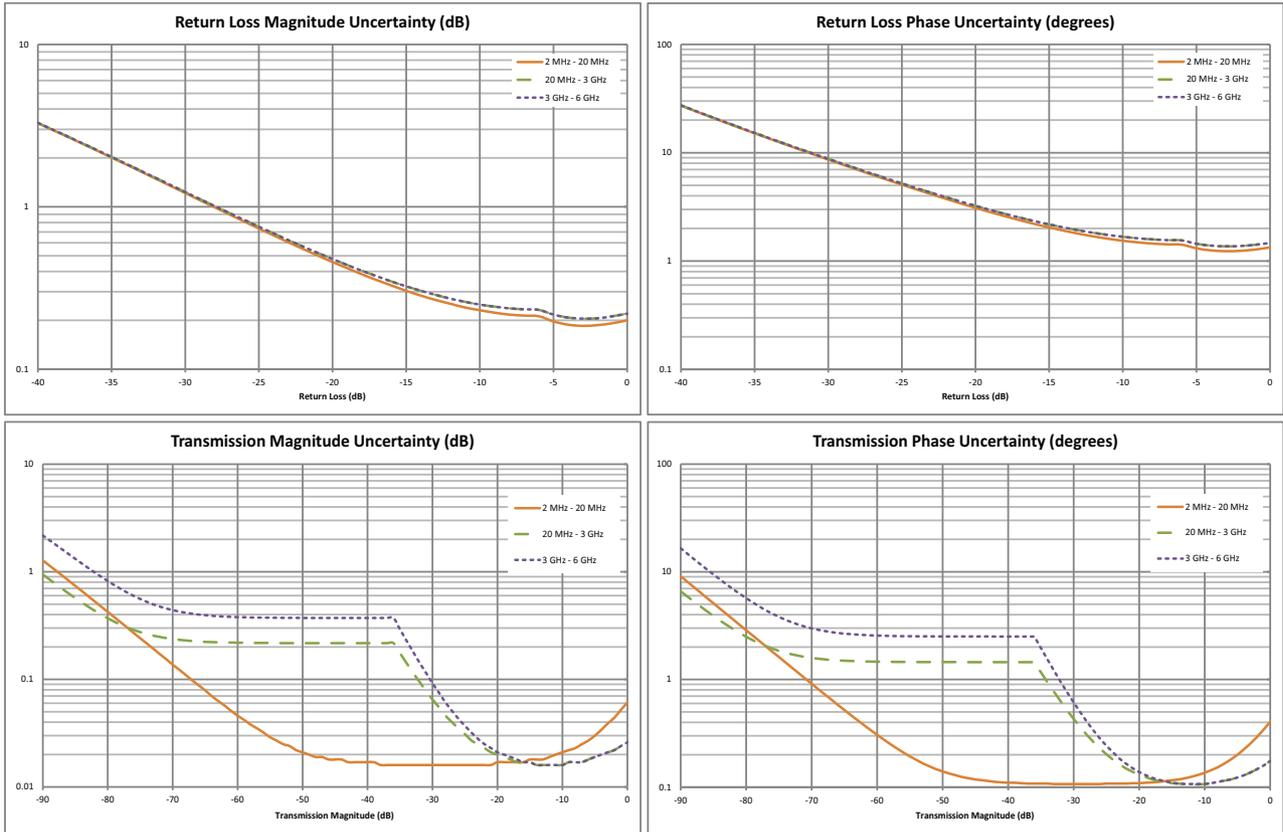
1. Full 1-path, 2-port forward path calibration with isolation, high power, 10 Hz IFBW, no averaging, 10 minute warm-up. OSLN50A-8, OSLNF50A-8, TOSLN50A-8, or TOSLNF50A-8 calibration kit. Reflection and Transmission Tracking are typical.
