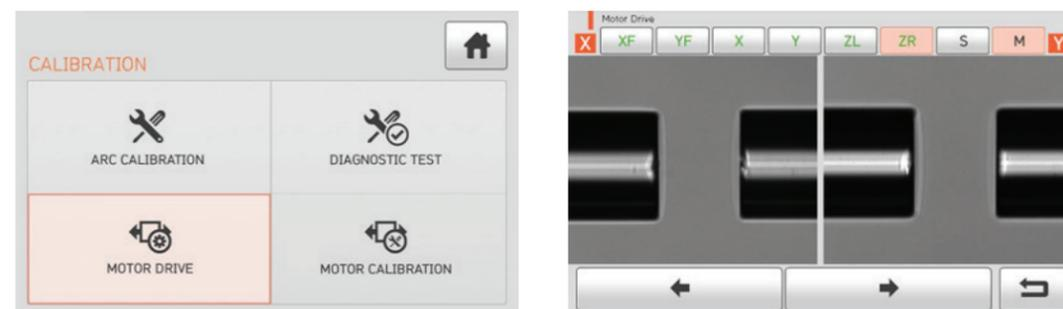
Selecting Motor Drive enables the user to manually test the motors on the K33A and ensure they are working properly. Motor Drive test requires the user to place fiber in the splicer.
