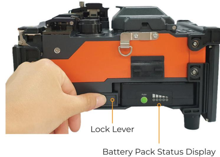
The unit be powered off before removing the battery to avoid damage. Remove the battery by releasing lock lever.
