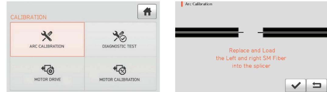
Below is what the screen will display while the arc calibration is being performed. The Arc Calibration will arc multiple times during this procedure so be sure to wait for the "Calibration Completed" message as seen below.
