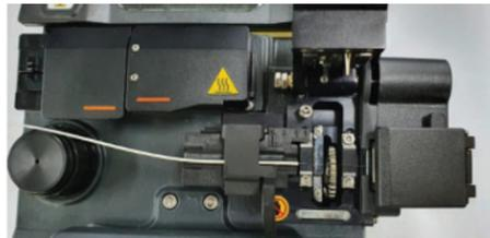
Press the cover to cleave the fiber and push the button on the self-rotating blade cleaver.
