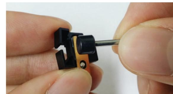
Replace the electrode blocks into the fusion K33A.
