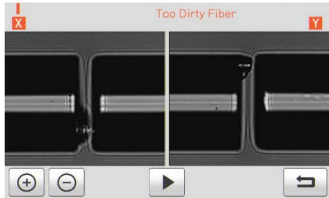
Replace the optical fiber. This message is displayed when the fiber is not correctly situated in the middle of the electrodes and V-groove or the optical lenses are dirty or obstructed.
