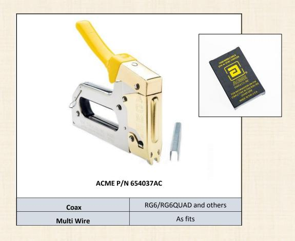
Model 37AC IS designed to drive the specially configured staples to a pre-determined depth in most substrates, thus making it virtually impossible for the Broadband wires to be crushed.
