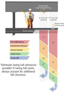
**Swing Falls:** Prior to installation or use, make considerations for eliminating or minimizing all swing fall hazards. Swing falls occur when the anchor is not directly above the location where a fall occurs. Always work as close to in line with the anchor point as possible. Swing falls significantly increase the likelihood of serious injury or death in the event of a fall.
