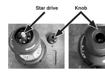
Place knob on the star drive and tighten the M8 to 2Nm (18 in lb).
