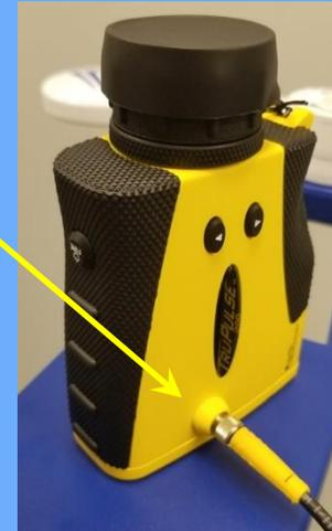
4. Hold the Laser at mid-height of the antenna and aim to the ground. The Laser does not have to be perfectly vertical, but it has to measure to an area at the same approximate elevation as the base of the tower.
