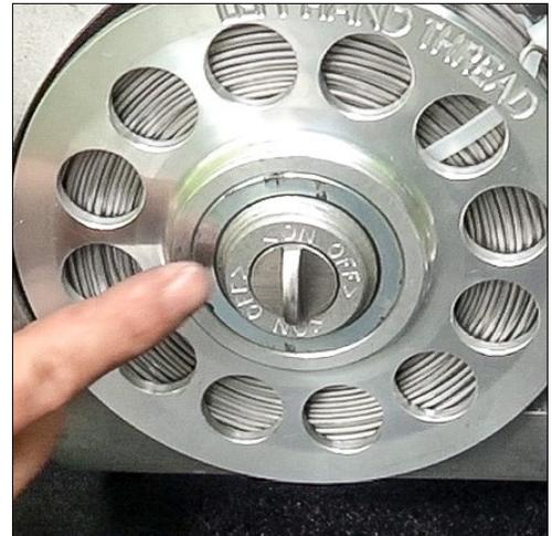
1. Once the lashing wire is loaded onto the Super G lasher, it is time to route the wire through the machine for proper operation. Pull enough wire off the reel to make the termination of the wire to the strand. Pass the wire under the tension adjustment roller then over the guide roller.
