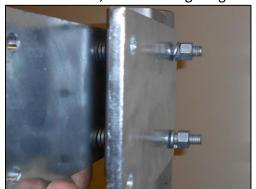
C) Install tube reinforcement in head assembly
