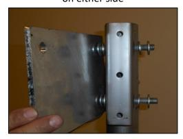
B) Finish connection with nuts and lock washers, attached finger tight
