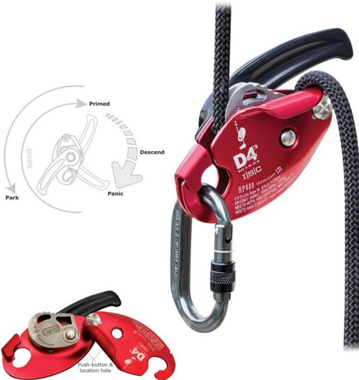
The new D4 Work/Rescue Descender features a unique and innovative progressive cam action which offers precise control at slow or fast speeds. The progressive cam works by way of one cam operating inside another cam, to provide a mechanical advantage and smoother control. The D4 is double-stop device with an auto-lock function whenever the operator lets go of the handle.
