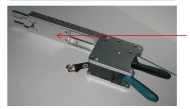
**1.** Place the AIR 32 Insert as shown into the Universal Mounting Bracket channel
