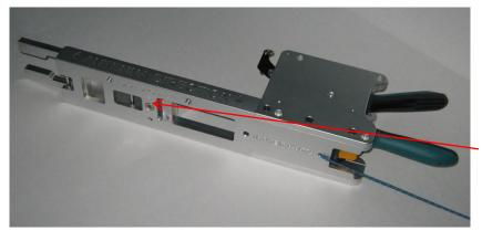
2. On the other side of the Universal Mounting Bracket insert the ¼-20 screw into the hole and screw tight. You should see it line up with the threaded hole on the Insert
