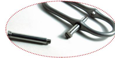
**6** To assure the pin is engaged properly, try to back out the pin using very light pressure- if there is resistance felt the pin is engaged properly, if not remove the pin and install a new one.
