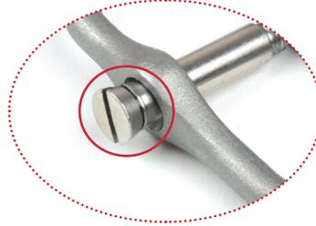
**1** The Double Dee rings are for the use on tools with enlarged ends only. Verify the C-Clip is installed on the pin prior to installing. It will fit loosely around the pin groove.
