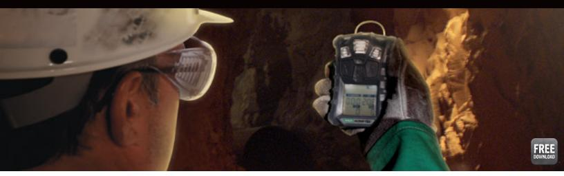
A gas monitor, also referred to as a gas detector, is a device that detects the presence of gas in an area. The device has sensors in it that are programmed to detect the presence of specific gasses. If that type of gas is detected, the gas detector will alert the user via an alarm. The most common sensors used in at-height, industry, and construction are:
