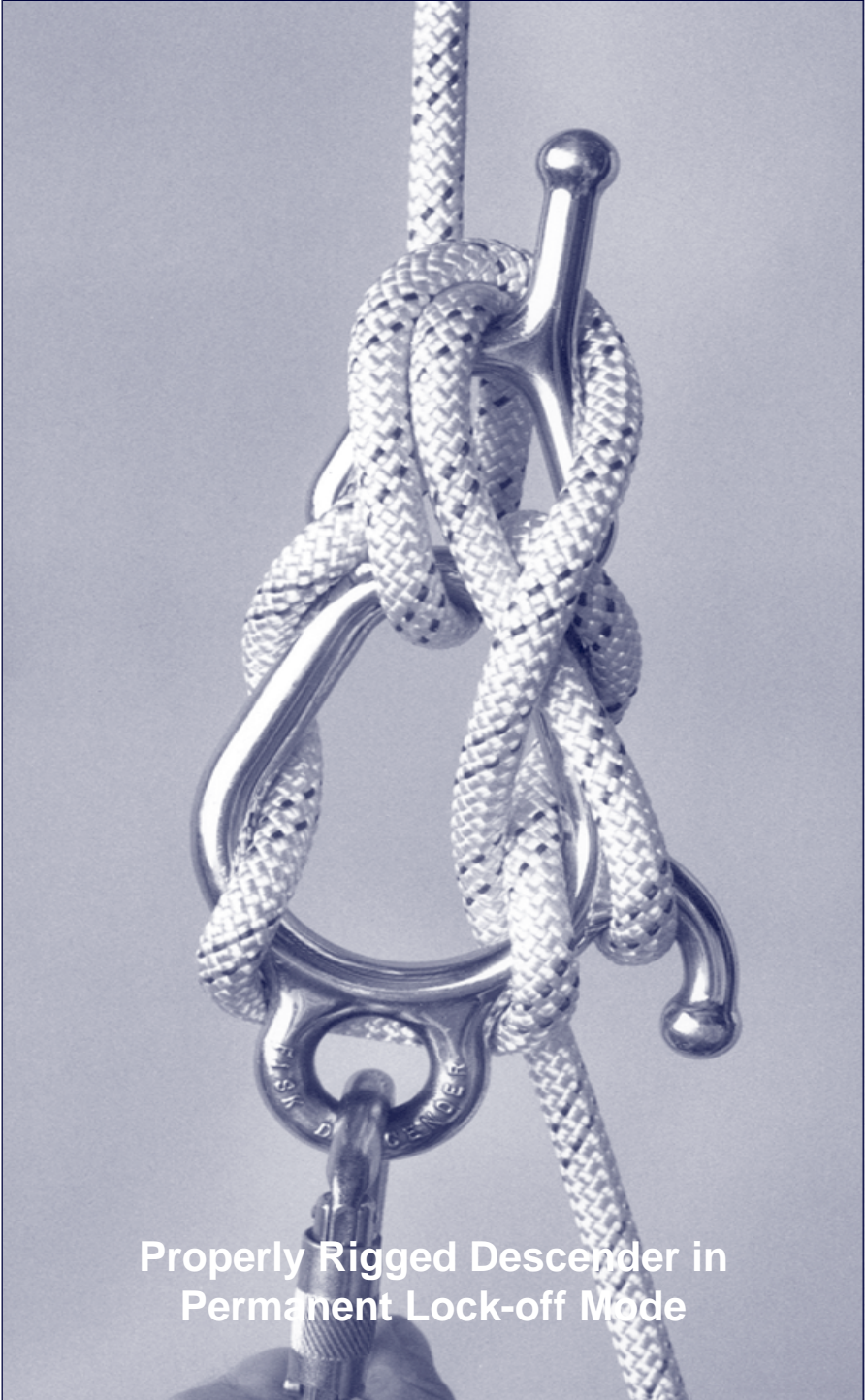
Figure 21 - Permanent Lock-Off Completion
