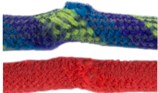
Pictures above showcase damaged rope cores and frayed/abraded sheath
