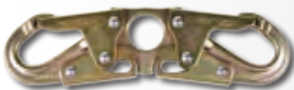
WESTFALL PRO SEPARATOR SPREADER BAR SNAPHOOK 9-3/4" x 2-1/4", 3/4" throat opening, 22.2 kN, double locking snaphooks, ANSI compliant. 07475 - $34.99
